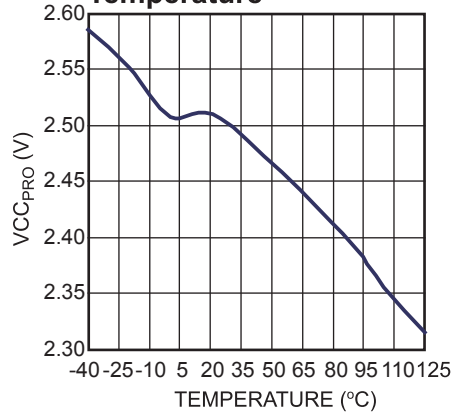
VCC Decreasing Level at which the Protection Phase Ends vs. Temperature
