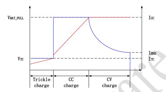
The battery target voltage can be set by KEY/BSET pin. When KEY/BSET is pulled up to VCC with a  $10 \text{K} \Omega$  resister, 4.2V is set; when selecting a  $15 \text{K} \Omega$  resister, 4.35V is set; when selecting a  $5.6 \text{K} \Omega$  resister, 4.4V is set; when selecting a  $3 \text{K} \Omega$  resister, 4.5V is set.
