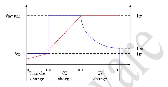
The battery target voltage can be set by BSET/HLED pin. When BSET/HLED is floating, 4.2V is set; when connecting a  $62K \Omega$  resister to ground , 4.35V is set; when connecting a  $30K \Omega$  resister to ground , 4.4V is set; when connecting a  $10K \Omega$  resister to ground , 4.3V is set.
