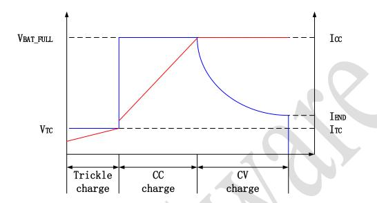
The battery target voltage can be set by BSET/HLED pin. When BSET/HLED is floating, 4.2V is set; when connecting a  $62K\,\Omega$  resister to ground , 4.35V is set; when connecting a  $30K\,\Omega$  resister to ground , 4.4V is set; when connecting a  $10K\,\Omega$  resister to ground , 4.3V is set.
